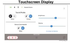
Select and drag down the Display & Audio Settings tab from the top of the screen. Voice status and Chime sounds can be enabled / disabled here. Blue indicates it is enabled. Screen brightness and volume can also be adjusted. Volume adjustment affects only Voice, Chime sounds, and Alerts. Alarm sounds are fixed and cannot be adjusted.
