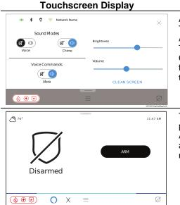
Description After the Alexa feature has been enabled on the Control Panel and each Touchscreen, the "Display & Audio Settings" screen displays a toggle button for Alexa Voice Commands on each enabled device. If Alexa is not enabled on a Touchscreen, Alexa Voice Commands are not displayed here. When Alexa Voice Commands is enabled, it turns blue and Alexa can be used with all available features. If disabled, Alexa cannot respond to any commands until it has been turned back on.
