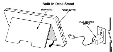
The Touchscreen can be powered by the supplied micro USB cable and the 5Vdc, 1.5A plug-in transformer. For optimal performance, use the supplied transformer to charge the Lithium Ion Polymer battery. The battery may not charge properly if it's plugged into any other USB port.
